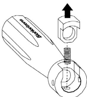
3. Release pressure from the button to remove the button and the button spring.
