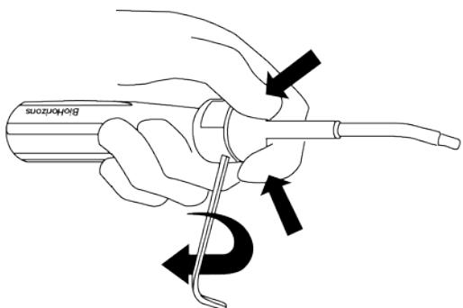
6. Hold the nozzle firmly against the handle with one hand and use your free hand to tighten the handle screws. Hand tighten using a 5/64" hex key.
