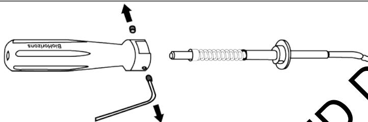
2. Keeping pressure on the button, slide the nozzle completely out of the handle. Then, remove the handle screws completely from the handle and set aside.
