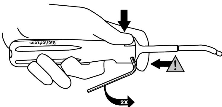
1. To release the nozzle from the handle, hold on to the flange of the nozzle as shown, maintain pressure on the button and slowly loosen the two handle screws approximately two full turns using a 5/64" hex key.
