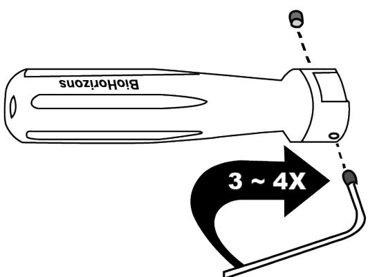
2. Pre-assemble the handle screws into the handle 1/4 full rotations.
