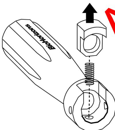
4. Carefully place the button spring into the small spring hole in the handle. Place the button on top of the button spring with the cut-out notch facing the firing end of the handle. Press the button down until fully seated and hold in place for final assembly.
